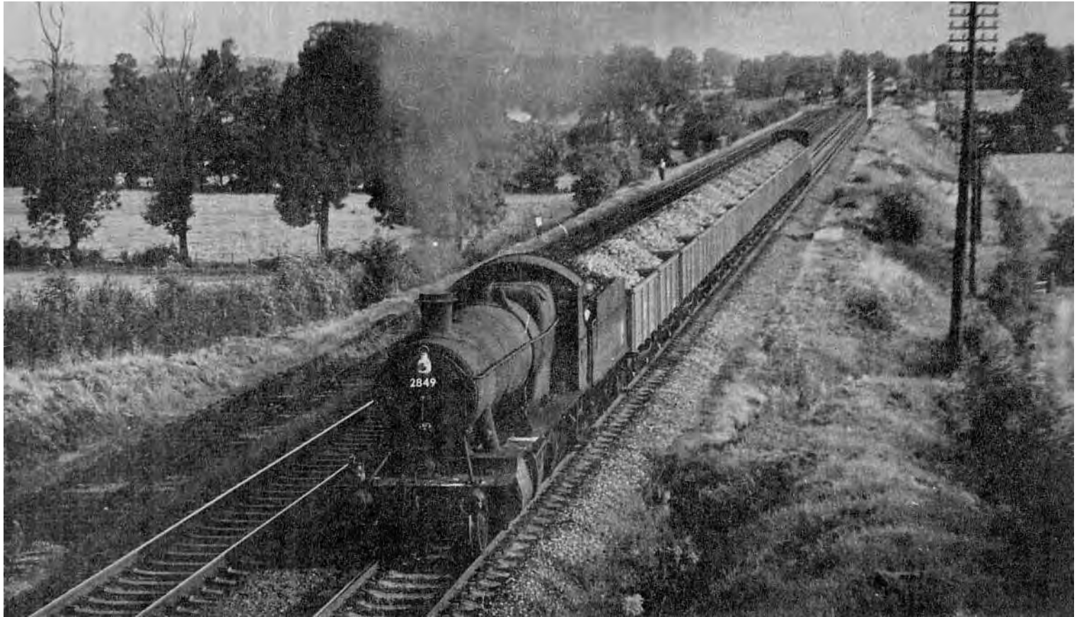
Fig. 9. A load of ironstone from the Oxfordshire Ironstone Company's quarries at Wroxton to South Wales by way of Fenny Compton, Stratford-upon-Avon and Honeybourne, is seen here on its way up Cropredy bank on July 31st 1961. The locomotive is an ex-G. W.R. 2-8-0 No.2849 of Newport (Mon.) shed, and the waggons are vacuum brake fitted tipplers. Already this is an historic picture. The ironstone quarries are now closed, and steam engines are no longer to be seen in north Oxfordshire.
